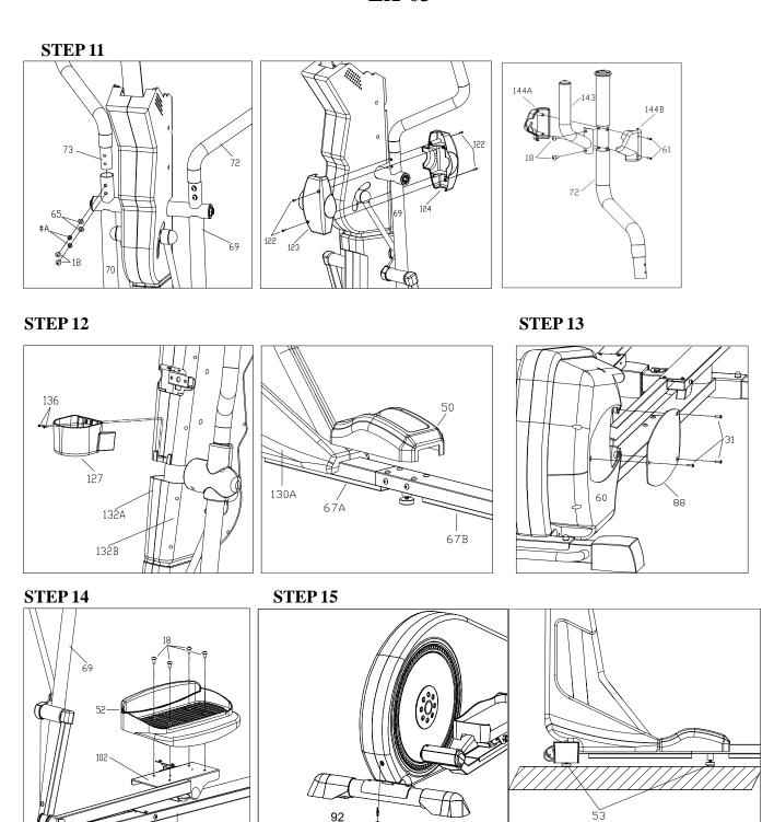
These are simple drawing to help to assemble the unit Detail of assembly please refer to the manual described.
